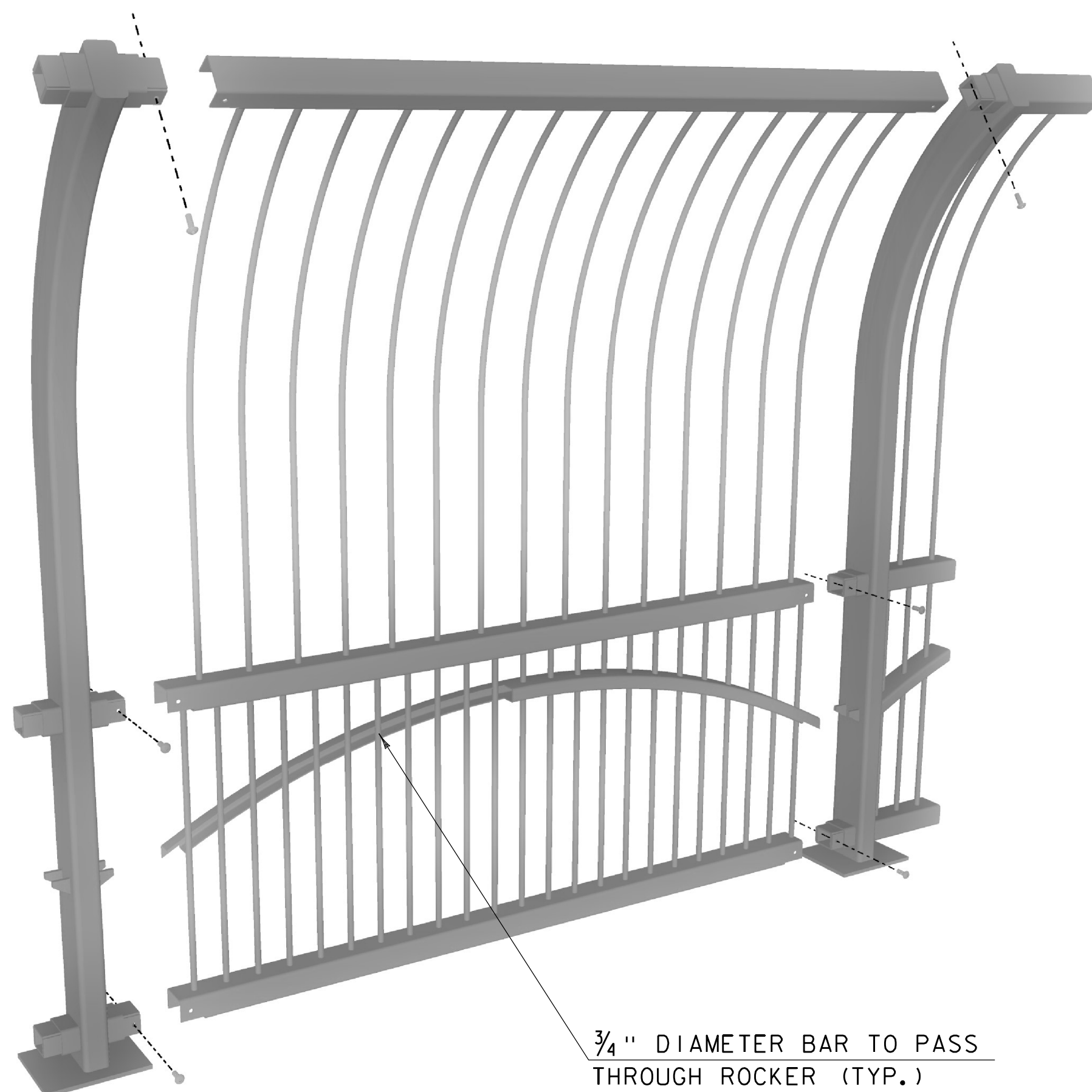
EXPLODED ISOMETRIC VIEW OF PEDESTRIAN SCREEN LIFT OUT PANEL SCALE 3" = 1'-0"
