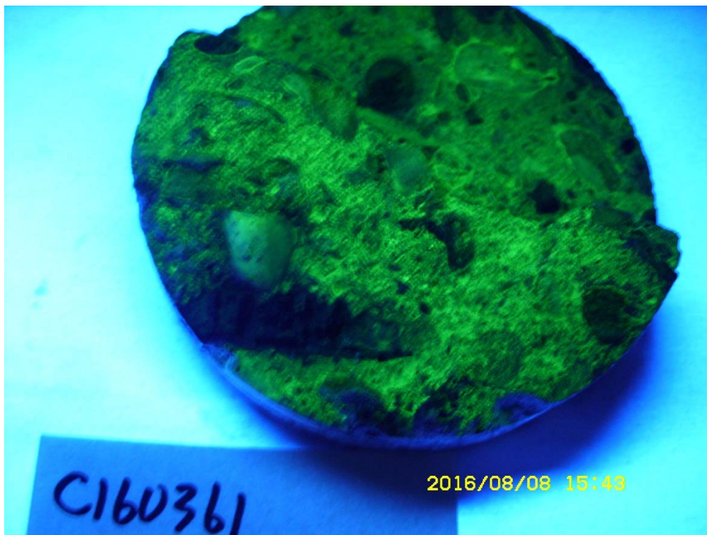
Core 1B from sample area 1, rated high ASR reactivity
