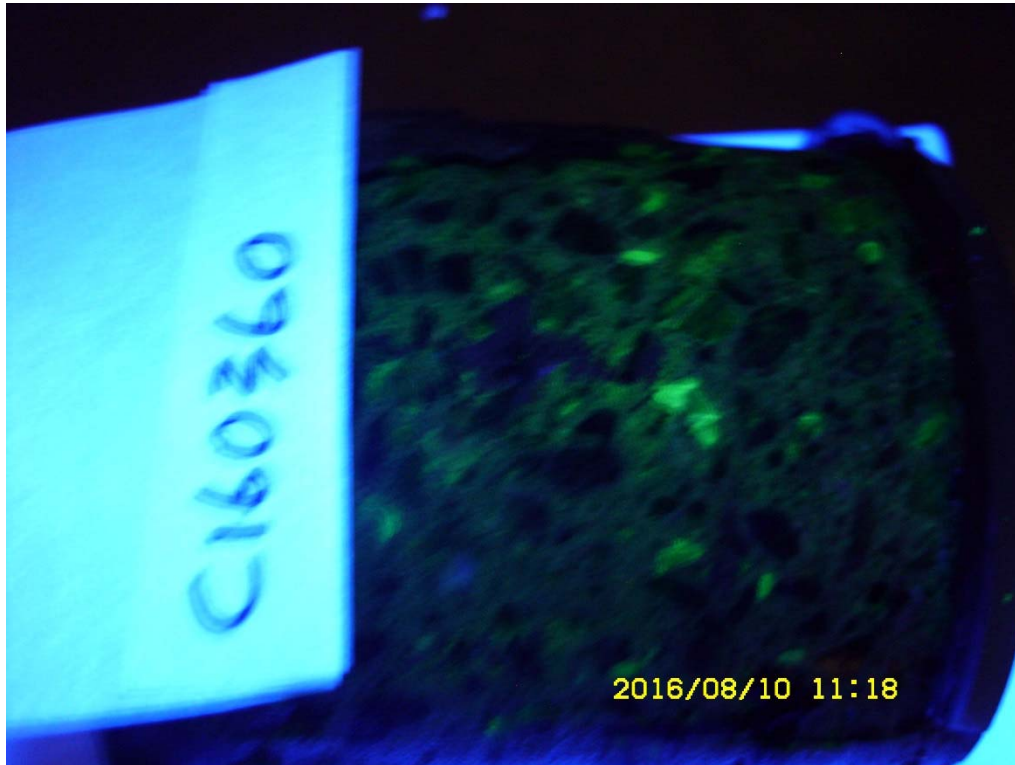
Core 1C from sample area 1, rated low ASR reactivity
