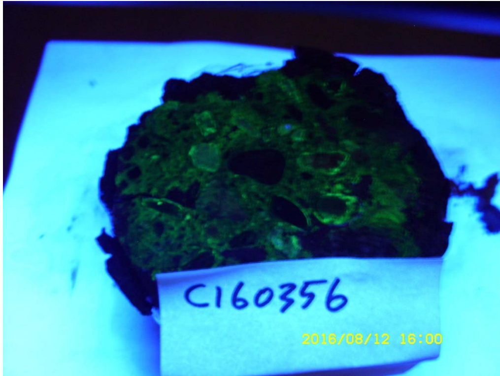
Core 1A from sample area 1, rated moderate ASR activity
