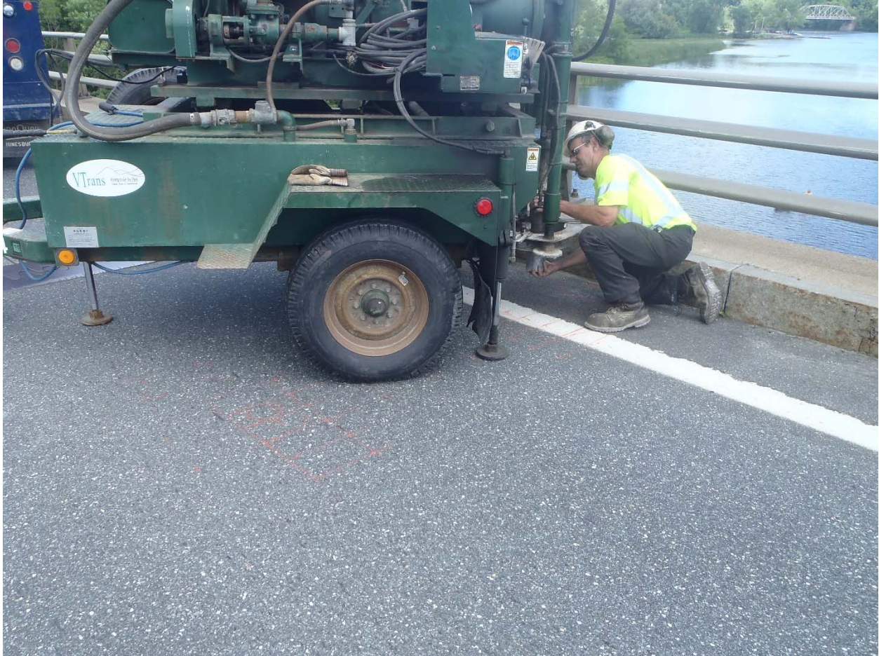
Trailer mounted core rig used by Vtrans Drilling unit used to cut the cores.
