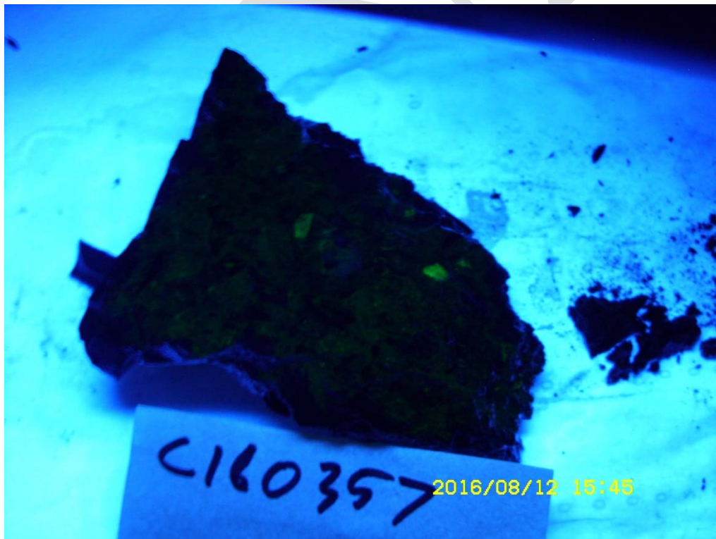
Core 2A from sample area 2, rated low ASR reactivity
