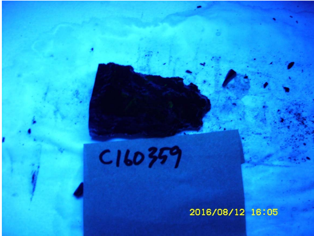
Core 2B from sample area 2, rated very low ASR reactivity
