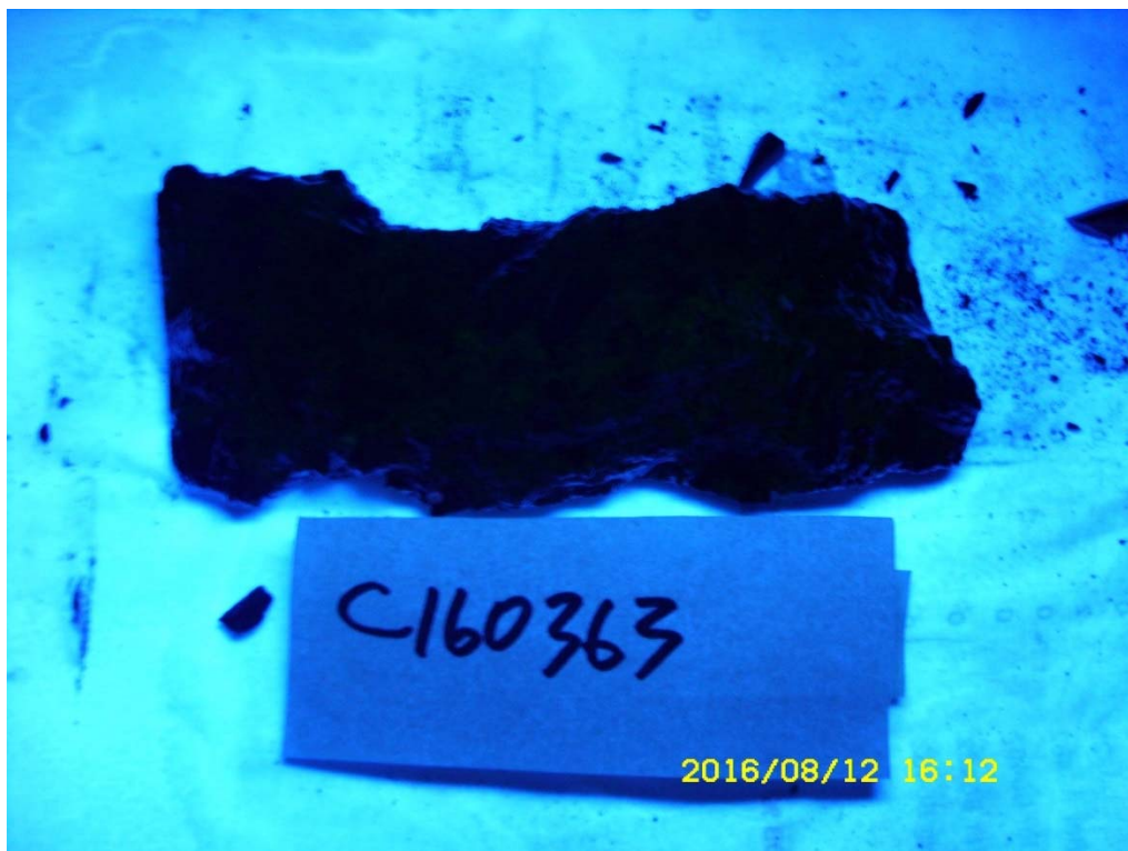
Core 2C from sample area 2, rated very low ASR reactivity
